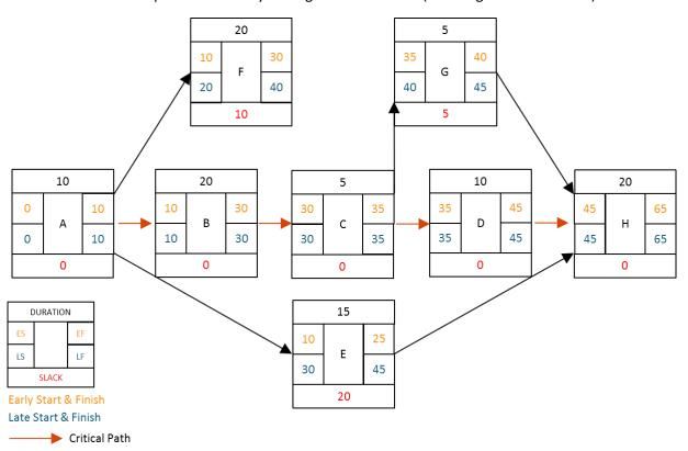
Figure 15.1: Critical Path Diagram
