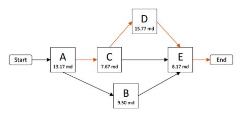
Figure 13.2: AON Network Diagram
