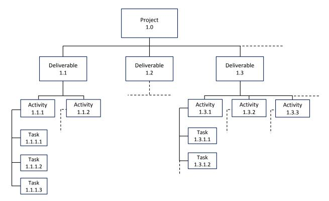
Figure 10.1: Work Breakdown Structure
